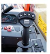
Joystick controller provides all the controls for convenient and enhanced operation of boom movements simultaneously and auxiliary boom end hydraulics. The controller is programmed to improve productivity.
