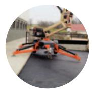
Boom orientation helps protect basket during towing (basket stows over the hitch side)
