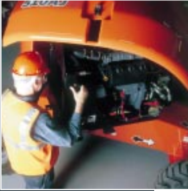
Swing out engine for ease of service
