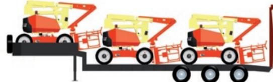
*Enables 3 machines to be transported on 12m trailer*
