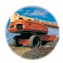
vvitn the tightest turning radius, best crab steer ratio and only oscillating axle in its class, you can go where other boom lifts simply can't.
