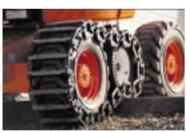
Semi-track Option with Floating idler Assists when travelling
