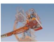
Articulating Jib\* Allows for greater versatility when positioning the platform around obstacles. \* Model 450AJ only.
