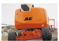
**Oscillating axle option for tough travel** Provides increased traction when travelling.
