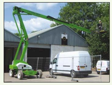
The HR21 Hybrid AWD also incorporates Niftylift's new ToughCage technology. Its touah impact resistant composite base and larger cross-section steel cage give extra strength and durability, both protecting the operator and reducing the risk of damage to the cage.
