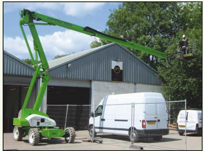
The **HR21 Hybrid AWD** also incorporates Niftylift's new **ToughCage** technology. Its tough impact resistant composite base and larger cross-section steel cage give extra strength and durability, both protecting the operator and reducing the risk of damage to the cage.
