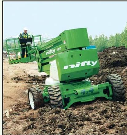
The Nifty HR17's unique suspension system ensures maximum traction when travelling over uneven ground and the 1.8m wide platform allows the operator ample space for tools.
