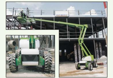
The unique suspension system shown above ensures maximum traction when travelling over eneven surfaces and the spacious 1.80m wide platform allows the operator ample room for tools and materials.
