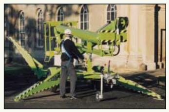
Fully proportional hydraulic outriggers make setting up and levelling quick and easy even on gradients.
