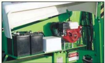
Petrol / Battery Bi-Energy power option, mounted for easy maintenance access. This system allows discreet and fume free operation or continual use even where an external power source is not available.
