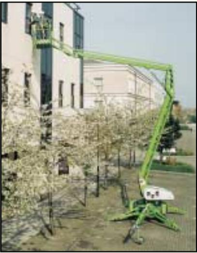
Hydraulic outriggers allow quick and easy setup and the unique talking alarm ensures that the operator is aware of an incorrect setup, even when working in the busiest of environments.
