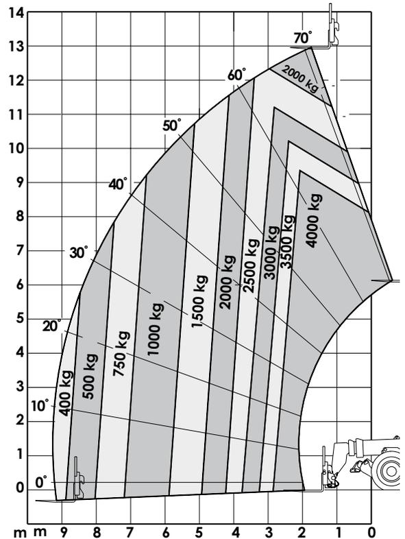
Frame levelling device activated.
