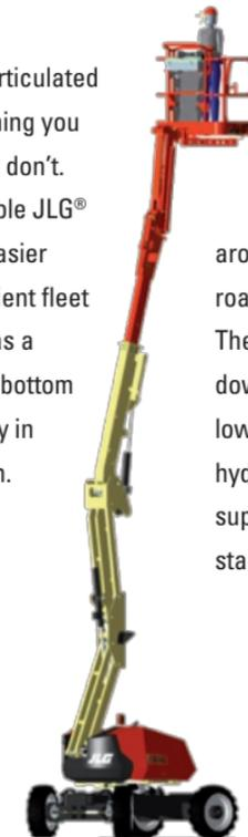
The 340AJ offers new standards in performance. Equipped with standard 4WD with oscillating axle, the 340AJ enables you to move around on any terrain, the on and off-road performance is excellent. The variable speed option and gravity down function of the boom help lower fuel consumption and efficient hydraulics saves on maintenance and supports modern working environment standards.
