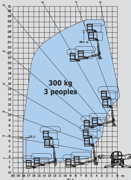
ROTATION ON STABILISERS FULLY EXTENDED WITH AERIAL JIB PLATFORM
