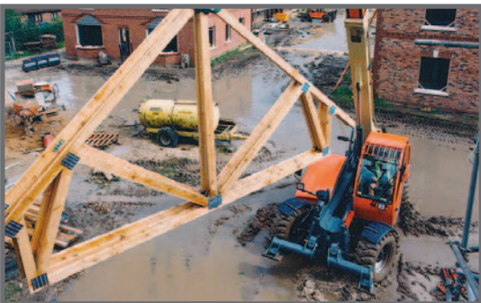
Truss Boom Nominal capacity 1,000 kg Allows the operator to position roof trusses, structural panels and formwork.
