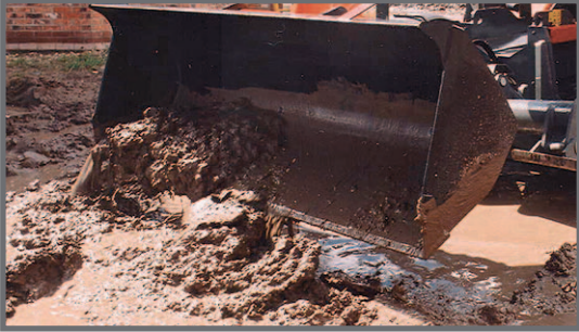
Digging Buckets Max capacity 1.0 m 3 Equipped with removable teeth to provide ground penetration when excavation jobs are required.
