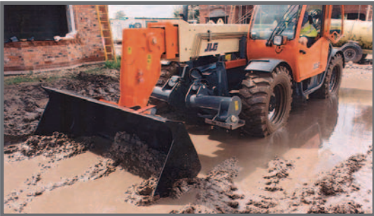
General Purpose Bucket Max capacity 2.0 m 3 Full width, heavy duty, robust general purpose bucket suitable for an array of tasks including on-site clean up and loose material re-handling.
